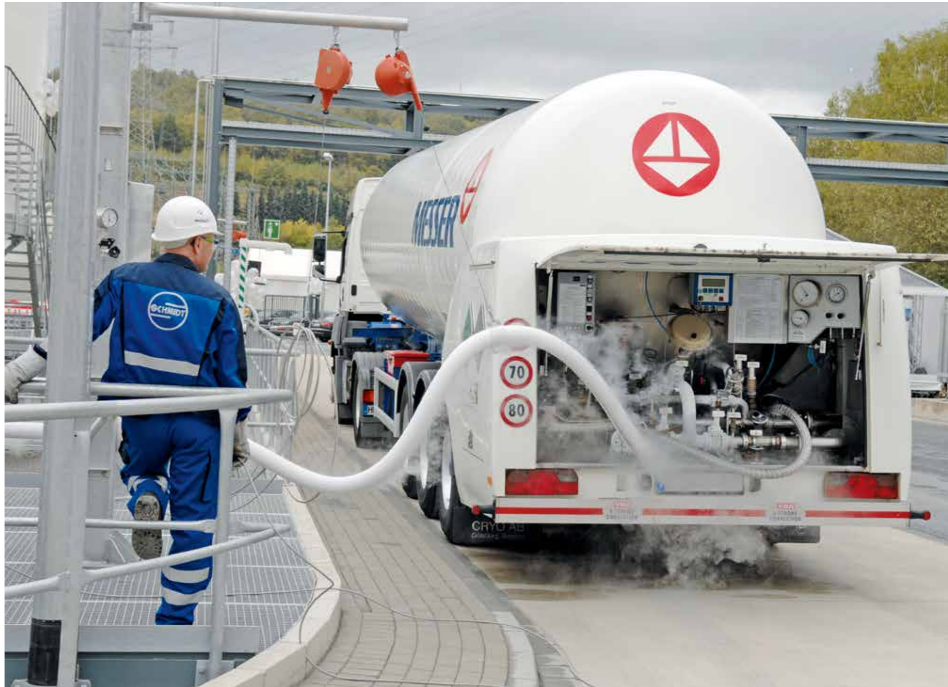
© Trailer unloading at Messer in Germany with a Hydran C-25/G2/HM
