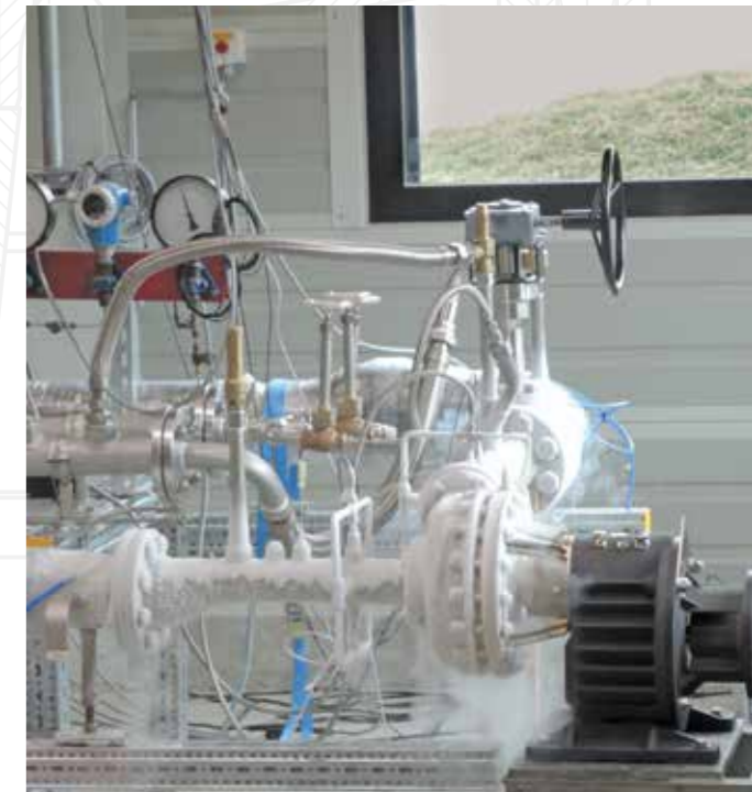
© Hydraulic and cryogenic test on fully automated LIN testing bench for ALL pumps
